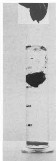
Concrete containing antiwashout admixture
